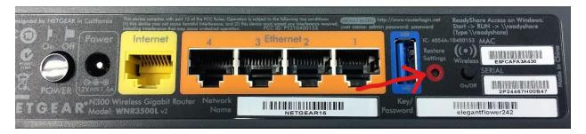
This is the last test you should try because it resets your router to factory default as if its brand new out of the box. If you do this then you will have to run the router set up again. If you had any custom settings – like router broadcast name or password – then you will have to reconfigure them. In most cases this is the ultimate fix.
