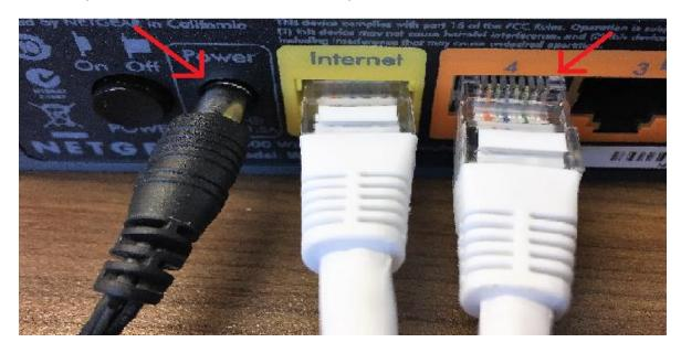
This may sound like a no-brainer, but we sometimes forget to check the most obvious solution before moving on to more complicated ones. Someone may have accidentally pulled on or kicked a cable causing it to unplug or become loose. You should check all of the cables involved and ensure that they're securely connected.
