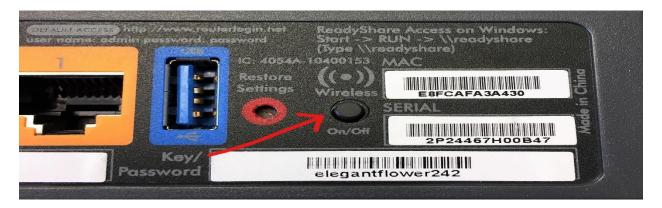
Most routers will have a wireless button on the outside of the router that can accidently get pushed and turn off your wireless.
