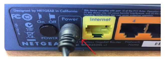
Remove the power from the back of the router and leave it unplugged for at least 10-15 seconds, then plug back in. Wait 5 minutes for the router to fully load back up and test your internet. This shouldn't be necessary, but some routers seem to need an occasional reboot to keep working well.
